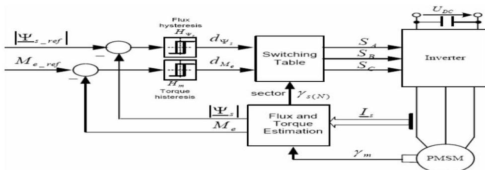
Figure.1. Basic DTC scheme
