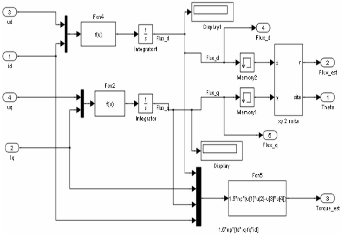
**Figure.8. Torque and flux estimator in PMSM**
