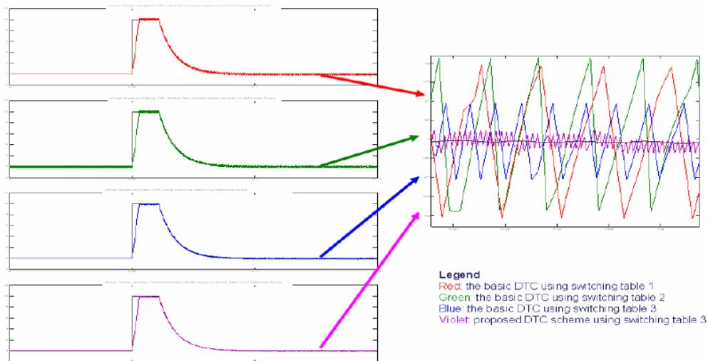
Figure.12. Comparison of the electromagnetic torque response under the basic DTC using switching table 1, using switching table 2, using switching table 3, and under proposed DTC scheme
