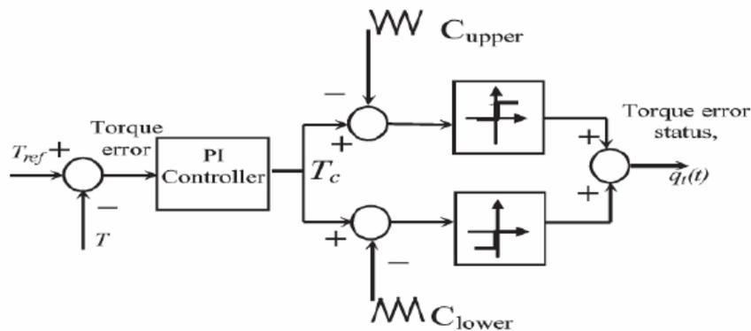
Figure.5. Torque Controllers
