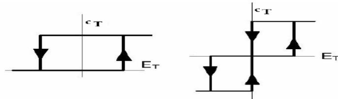
**Figure 3 Two and three level torque hysteresis controller characteristics**
