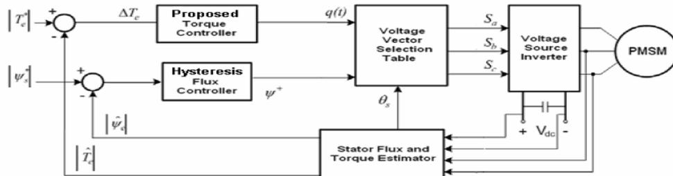
Figure.4. Proposed DTC Scheme
